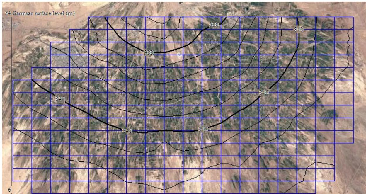
*The Garmsar alluvial fan (Google Earth) overlain by the SahysMod nodal network (blue lines) and the surface level contour lines (black) made with the QuikGrid program.*
