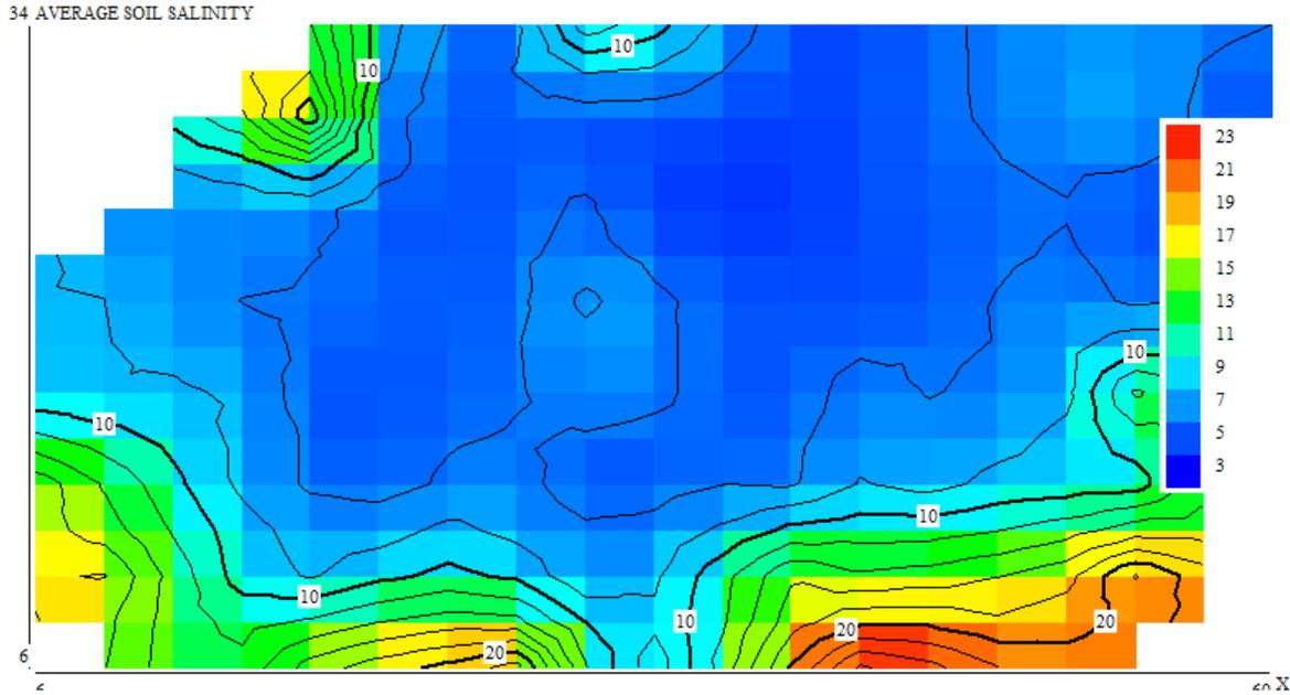
Contour lines of soil salinity with the same data as in the foregoing illustration. The map is made with the free Quikgrid program.
