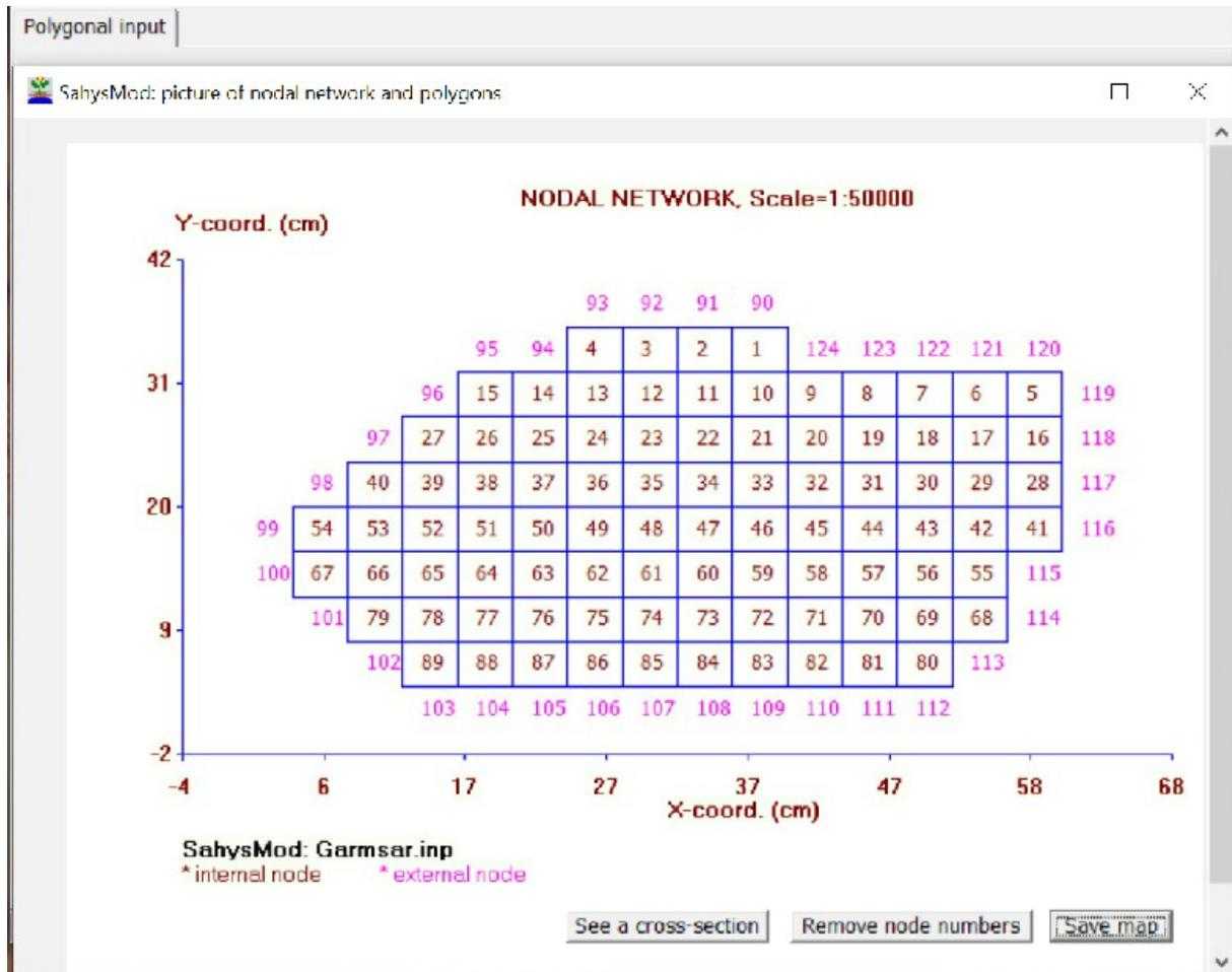
Figure 6. Picture of map of the network of the polygons. There 89 numbered internal polygons (blue) and 35 external polygons defining the boundary conditions (purple numbers) making a total of 124 polygons. The map gives the possibility to “See a cross-section” over those polygons in a straight line wanted by the user. It is also possible to reduce the size of the network with the “Remove node numbers” button.
