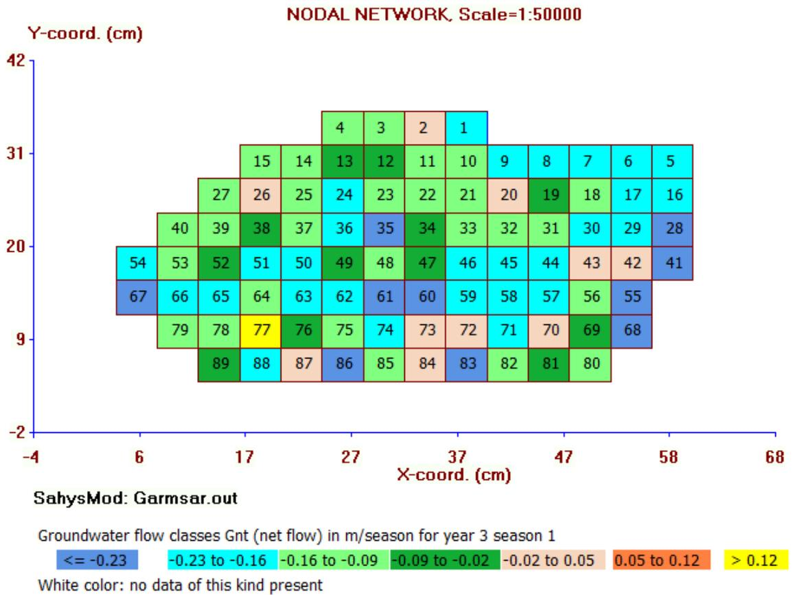
Figure 20. Polygonal map of the net groundwater flow (Gnt, incoming flow through aquifer and transition zone from neighbor polygons into the central polygon less outflow through aquifer and transition zone from the central polygon to neighbor polygons).
