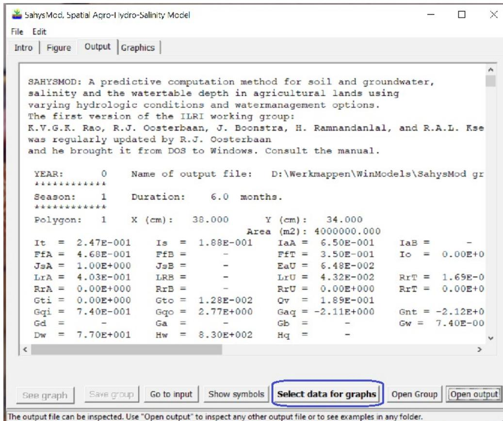
Figure 9. Overview of the top of the output file. The file can be further inspected using the scroll bars. The output file is quite big and its inspection is tedious. Therefore the possibility exists to inspect the output per group and see their graphs using the "Select data for graphs" button (blue square).
