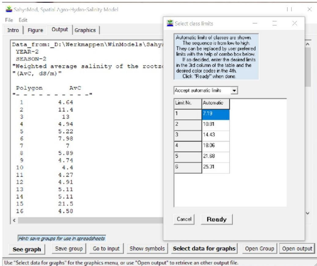
Figure 17. This figure is like figure 15, but is has an insert to the right, indicating that the map will be made automatically with salinity class limits as given in the table.
