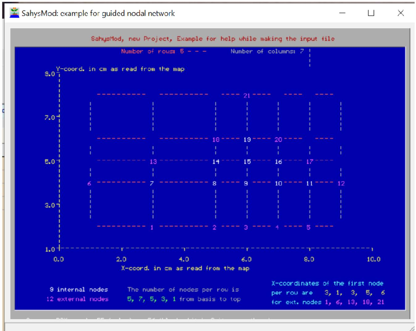
*From this figure one gets the impression how the horizontal and vertical grid lines are formed, how the horizontal X and the vertical Y coordinates are depicted and that there will be internal polygons, indicated by white nodal numbers, and external polygons, indicated by purple colored nodal numbers. The nodes are the centers of the polygons to be formed.*
