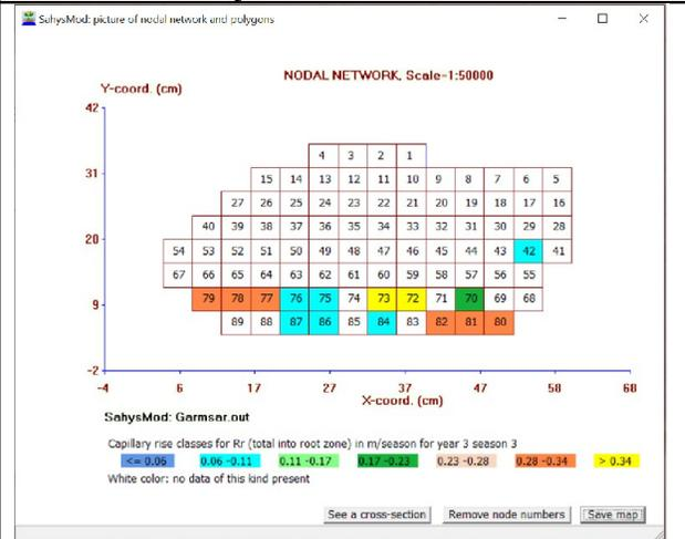
**The capillary rise of water from the underground into the dry root zone**
